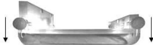
7. Place the tray in its place within the gel box, and pour in enough buffer so that the liquid level is about a centimeter above the surface of the gel tray. Wells should be oriented towards the negative (black) side of the gel box.
