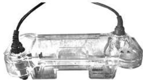
The red cable has the positive charge, while the black cable has the negative charge. Your DNA sample has a negative charge, so it will be traveling through the gel towards the positive charge as electrophoresis takes place.
